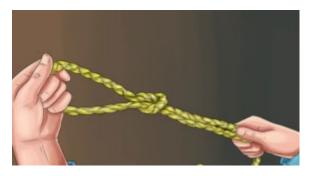
Once the 50 cm pieces are all cut and the ends are properly heat-sealed by the hot-knife, each piece of twine is made into a loop by knotting the ends together.
