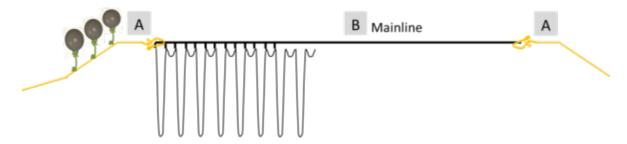
Figure 23 Schematic view of the mainline [B] attached to the loop of each unusable section [A] at each end, the longline is showing collectors attached at equal distance along the mainline
