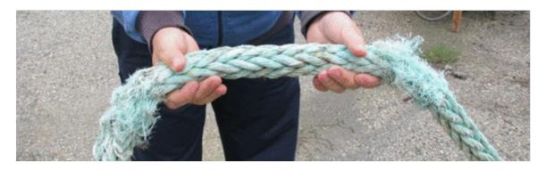
Figure 18 Consequence of using unknown rope material and mixing two rope qualities together
