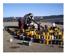
Figure 17 Production of compensation ballast weights
