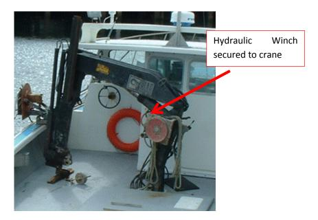
Figure 58 Hydraulic crane with the winch and controls
