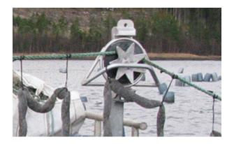
Figure 59: Starwheel set up on a mussel workboat
