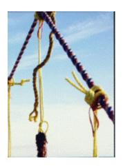
Figure 41: Dropper rope is passed through loop cord
