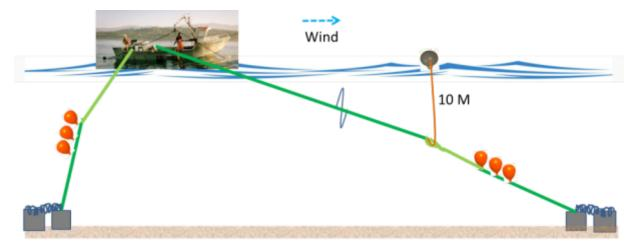
Figure 51 Tightening the longline
