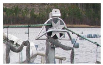
Figure 24 Mainline rolling through the starwheel
