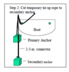
Figure 49 Concrete anchors deployment method for small water craft
