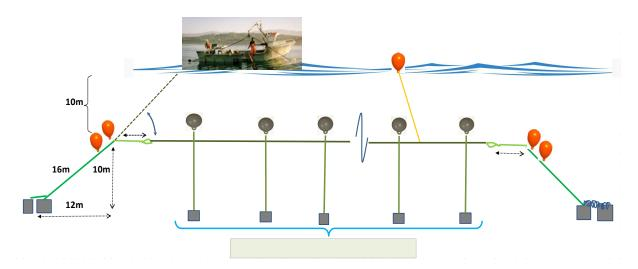
Figure 15 Schematic representation of submerged longline with evenly distributed intermediate floats
