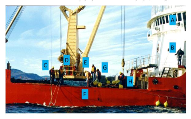
Figure 48 Deployment of the concrete anchors in a longline series from a big ship able to move 3 tons anchor
