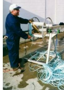
Figure 34 Rolling rope around spindle
