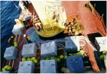
Figure 45 Preparation of longlines for deployment with big ship
