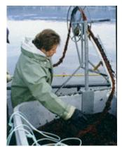
Figure 56 Hand-made mechanical wheel with a counter to measure collector rope length
