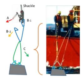
Figure 47 Anchoring
