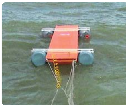
Figure 10: Floating device with installed linear movement generator.
